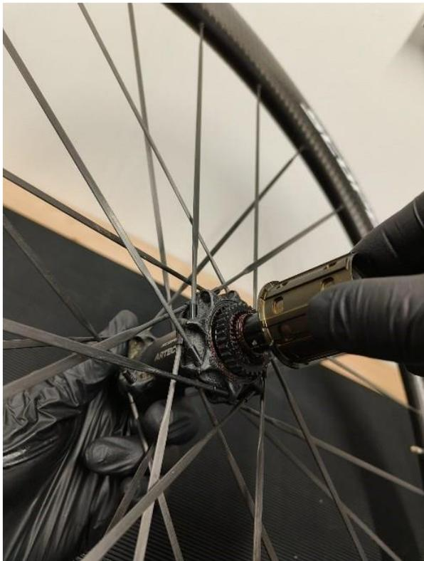
A photograph showing a person's gloved hand using a ratchet to attach a hub body to an axle. The ratchet is positioned on the hub body, and the axle is visible. The background shows the spokes of a bicycle wheel.                            |
