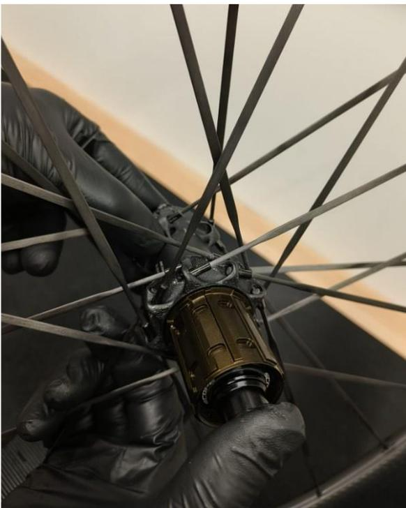
A close-up photograph showing a person's hand wearing a black nitrile glove. The hand is holding a cylindrical end cap and is in the process of sliding it onto a hub. The hub has several spokes radiating from it. The background is dark and out of focus.                   |
