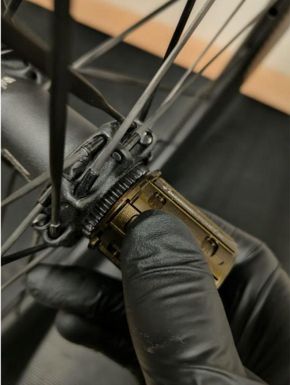
A close-up photograph showing a person's hand wearing a black nitrile glove. The hand is holding a large, silver-colored ratchet mechanism. The ratchet is being pushed or adjusted against a hub shell. The background is dark and out of focus, showing some mechanical parts. |
