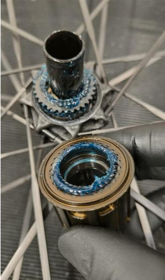
A close-up photograph showing a person's gloved hand applying a thick, blue grease to the teeth of a ratchet gear. The gear is part of a larger mechanical assembly, and the background shows the spokes of a bicycle wheel. |
