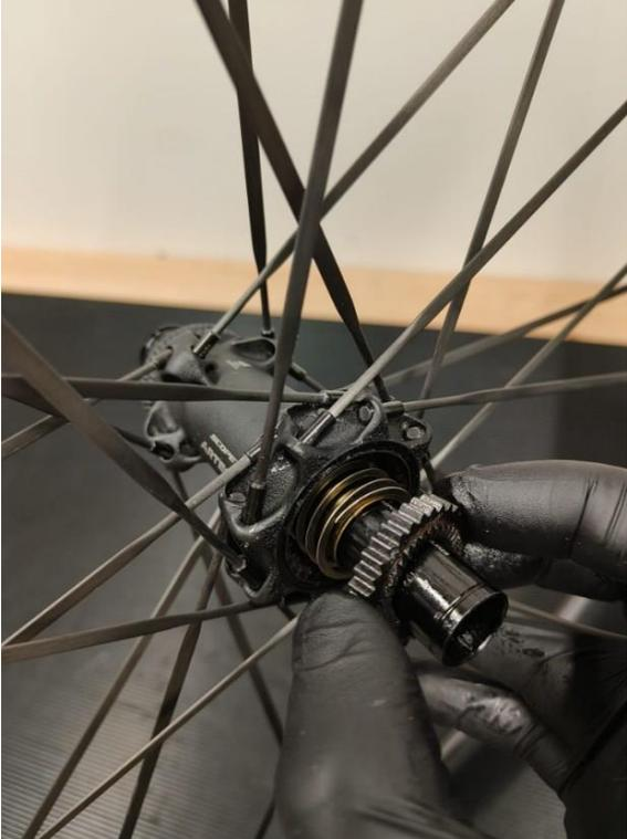
A photograph showing a person's gloved hand installing a large ratchet gear onto a hub shell. The gear is being pushed onto a spring mechanism. The background shows the spokes of a bicycle wheel.                         |
